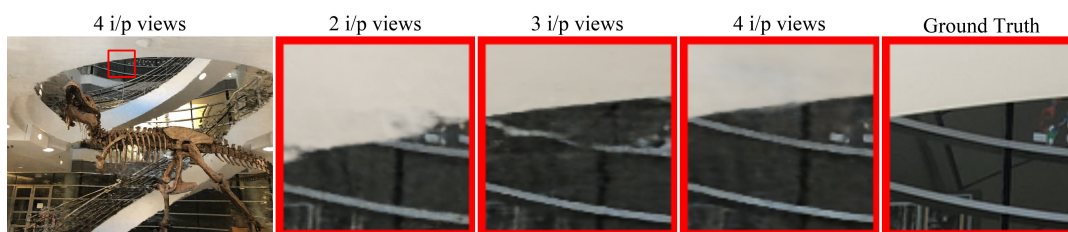
Figure 11: Qualitative examples on the LLFF dataset with two, three, and four input views. We observe errors in depth estimation with two input views causing a change in the position of the roof. While this is corrected with three input views, there are a few shape distortions in the metal rods. With four input views, even such distortions are corrected.
